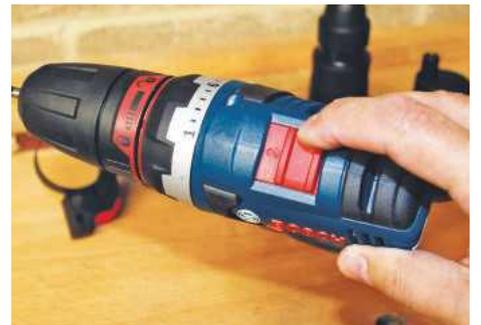
▲ The body has a standard 2-speed selector switch and torque collar
